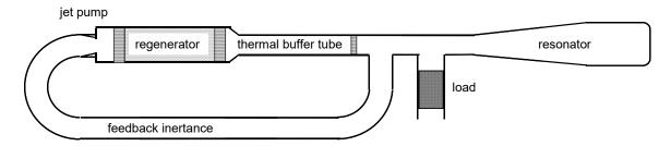
In the Sage model all the components arranged in the top-level edit window:
